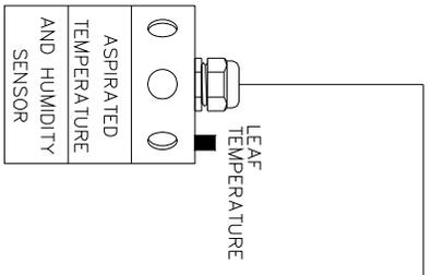
LOCATE IN THE CENTER OF CONTROLLED AREA AWAY FROM DIRECT CONTACT WITH GREENHOUSE METAL POSTS AND MEMBERS.
