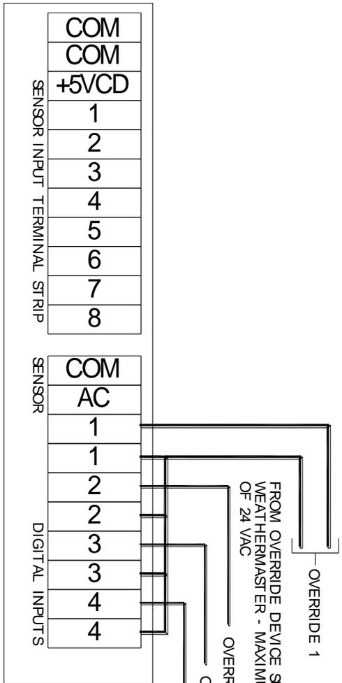
USE THE SAME CONFIGURATION FOR OVERRIDES 2, 3 AND 4. OVERRIDE 4 CAN ALSO BE USED AS PHOTOCELL INPUT.
